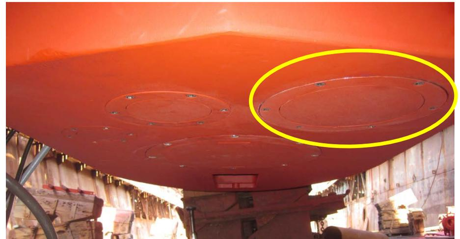
70 kHz transducer was added to cover the gap between 38 and 120 kHz.
